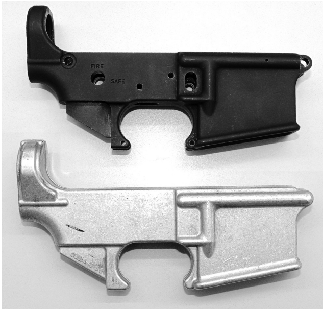
Figure 4.48 Regardless of whose name ends up stamped on the receiver as the manufacturer of record, most AR-15/M16 lower receivers start off as an aluminum forging (the same is true for the upper receivers as well). The example on top is ready to make operational and only needs the internal parts to operate; the forging shown on the bottom is the legal equivalent of a paper weight and is not considered a receiver at this stage of manufacture. AR receivers can be made of carbon fiber or other metals, but aluminum remains prevalent. (Image from author’s collection.)
